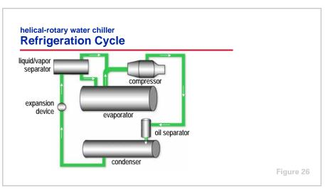
But first, lets review the components of the helical-rotary chiller's refrigeration cycle...
